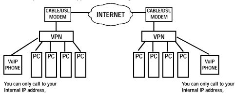
Setup Diagram D (Not Recommanded, Professional Installation Required) PI Gatekeeper does NOT support for this setting.
